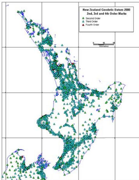
**Figure 2. North Island 2nd, 3rd, and 4th Order 2000 Geodetic Network**
