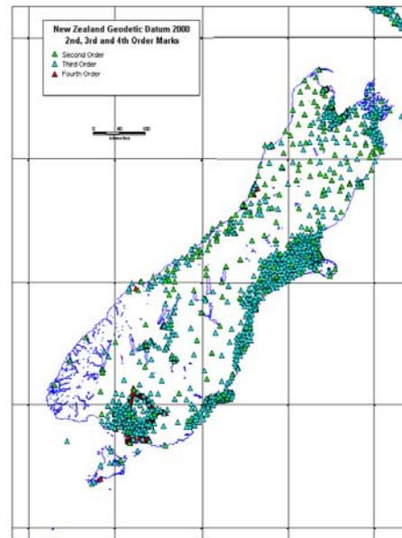
**Figure 3. South Island 2nd, 3rd, and 4th Order 2000 Geodetic Network**
