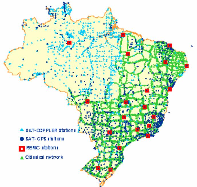
Figure 7 - Geodetic Network adjusted in 2006
