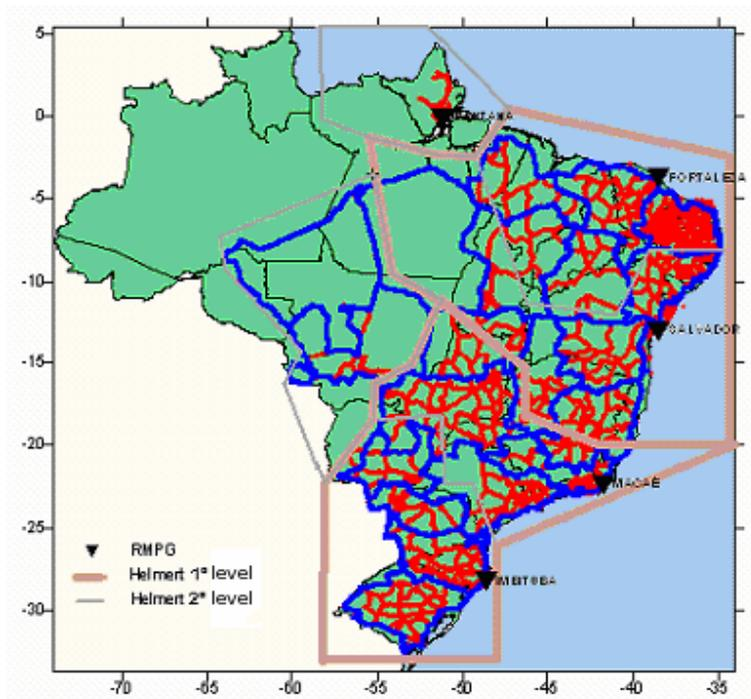
Figure 1 - Leveling adjusted network
