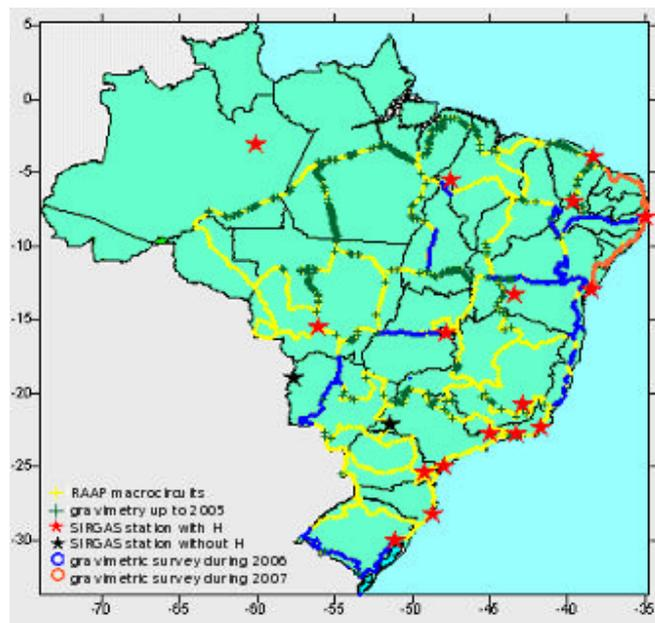
Figure 2- BMs surveyed with gravimetry in 2006 and 2007
